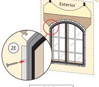
F. **Plumb and square window**. Place shims 1" from the bottom and top of the window between the window and the sides of the opening. Adjust the shims as required to plumb and square the window in the opening. If the frame height exceeds 53", place shims at the midpoint of the window sides.
